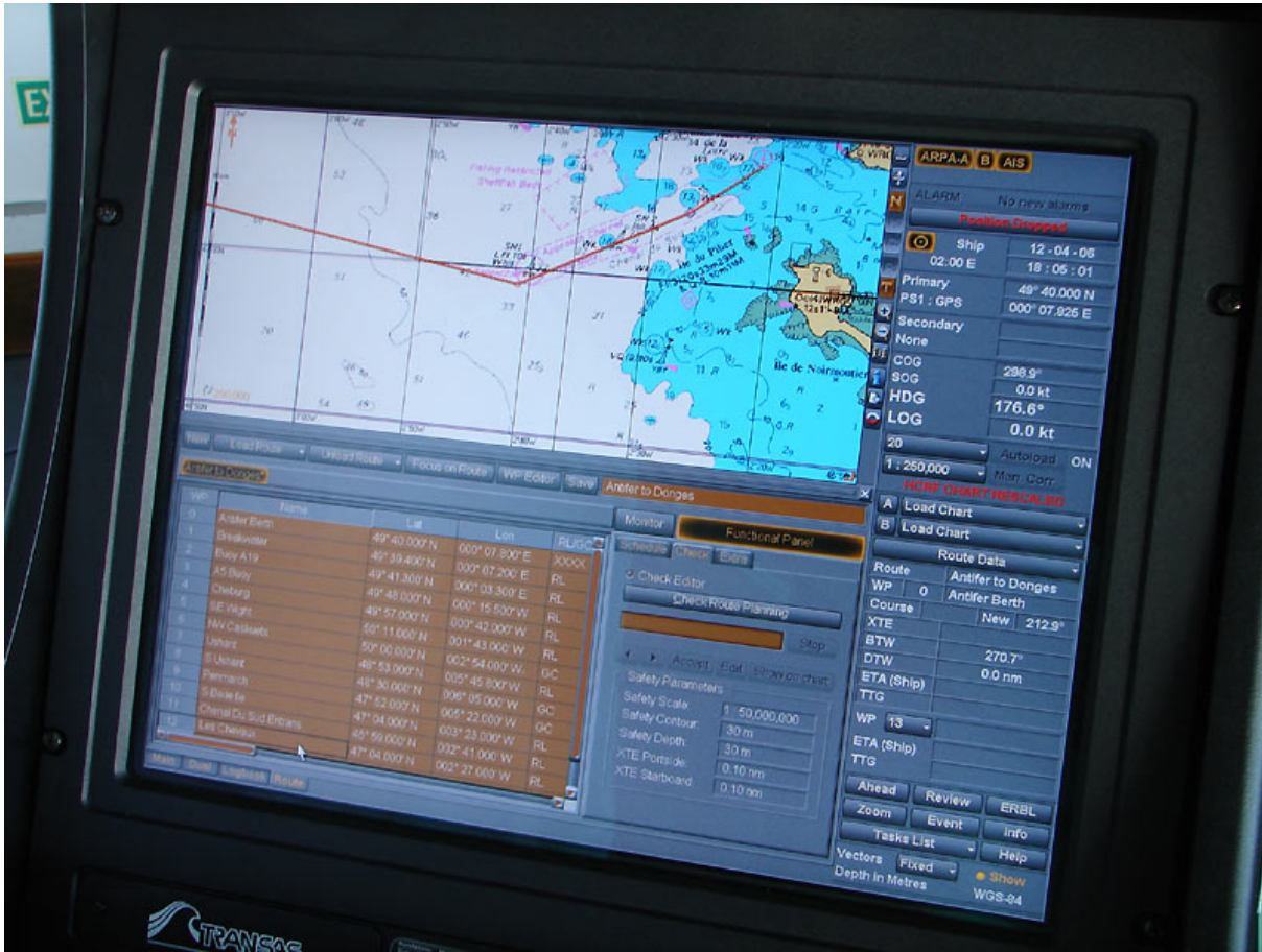
Figure III.7: Example of an ECDIS Human Machine Interface (source : Wikimedia Commons , unmodified picture, author: Hervé Cozanet , license : CC BY-SA 3.0 ).
