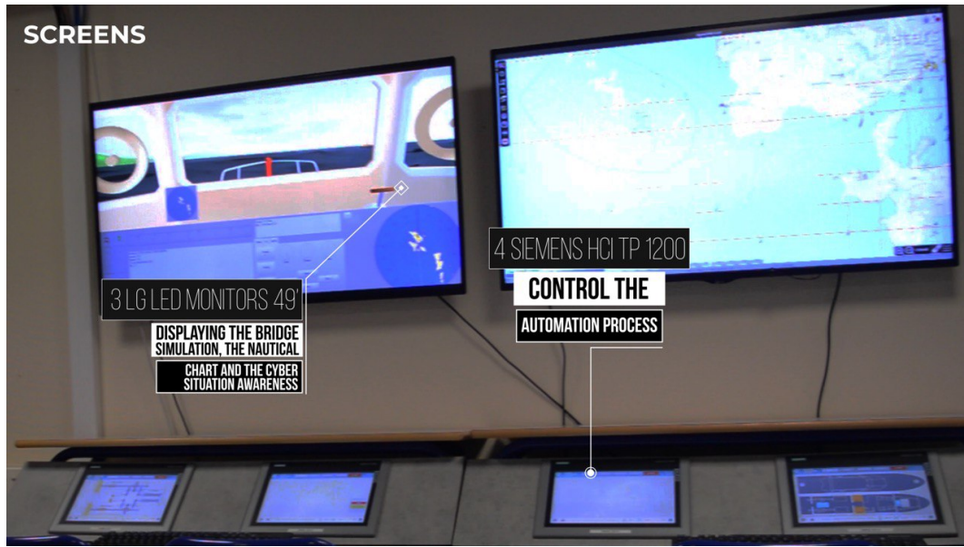
Figure IV.2: Simulation environment of the navigation bridge (source: Naval cyber defense chair , reproduced with the kind permission of the author).
