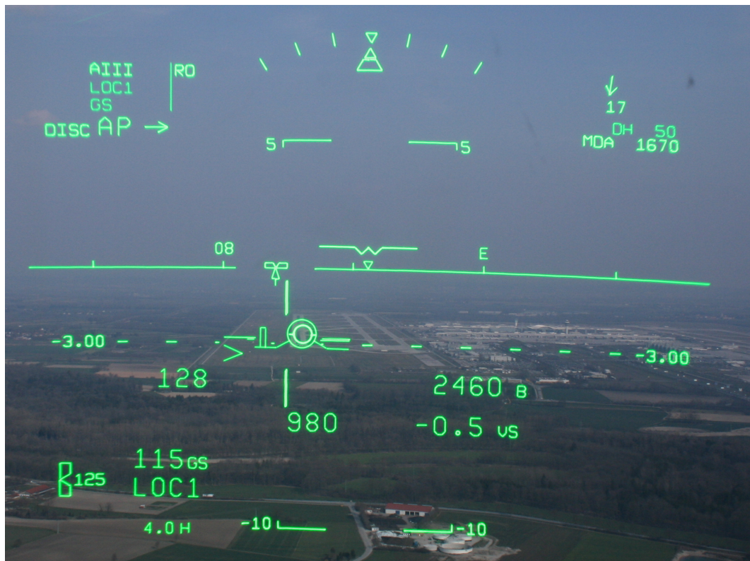
Figure III.5: Head Up Display of a Bombardier CRJ-900 passenger jet in long final at Munich airport (source: Wikimedia Commons , unmodified picture, author: Joschiki, license: CC BY-SA 3.0 ).
